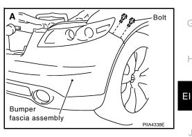
Insert driver rolled with cloth between bumper fascia and "S" type clips, and remove bumper fascia.
