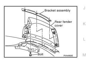
Remove bracket clips and remove bracket.
