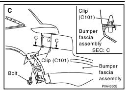
11. Remove bumper nuts and remove bumper stay. Remove nuts with power tool.
